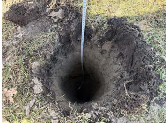
Image 12: Test pit to 1.20 m showing shallow topsoil and deep yellow beach sand. Facing north.
