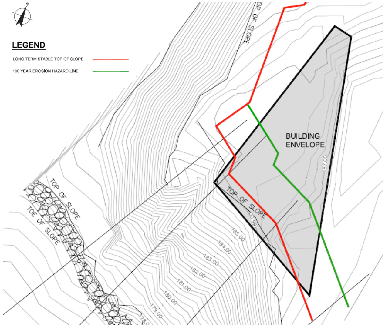
Figure 4 Long-Term Stable Top of Slope and 100-Year Erosion Hazard Line
