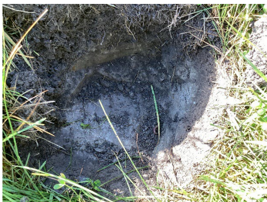
Photo 31: Sample Undisturbed Test Pit [4]
